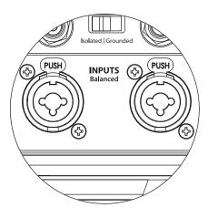
The Left and Right inputs on the Fathom IWSv2 are internally summed to a single mono channel. Since the Fathom IWSv2 is inherently a "mono" or single channel device, you can use the Left and Right inputs for the master Fathom IWSv2 and then distribute the summed mono signal to additional slave Fathom IWSv2s in the system.
