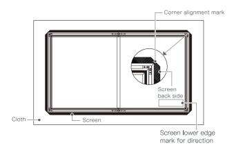
4. Fix the screen onto the frame with all the springs in order as indicated below (corners, short sides, then long sides).
