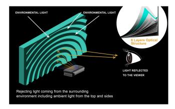
AWOL ALR rollable Fresnel daylight screen is equipped with 8 Layers optical structure to offer 4K&8K Ultra HD resolution, 3D capable, 1.1dB peak gain, 85% rejection ratio, neutral color temperature, and enhanced picture contrast in a theater, grade image.
