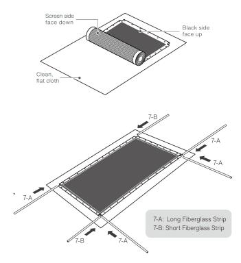
Put the assembled frames on the back side of the screen.
