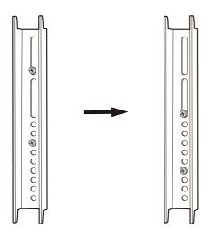
You can fine— tune the installation height of the screen without drilling new holes based on the screw holes in the upper wall bracket and the lower wall bracket spring range.(Adjustable height range: 0–2.0 inches)
