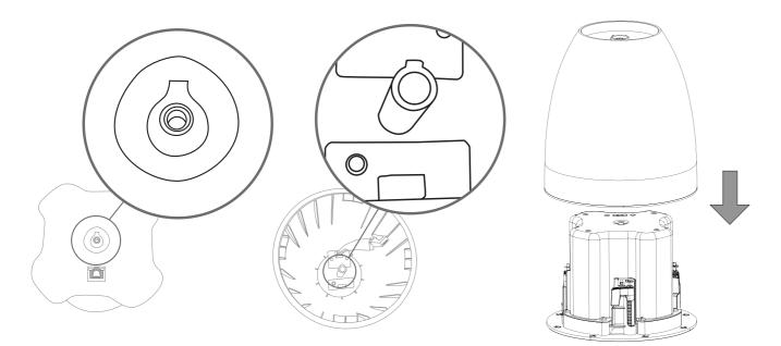
Install and fix hook screw with lock washer
