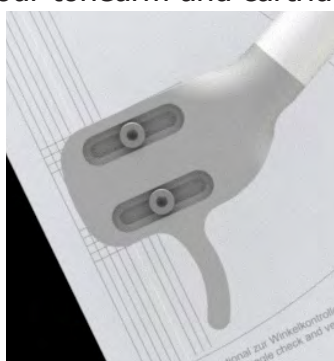
Pic. 2: Alignment of the cartridge
