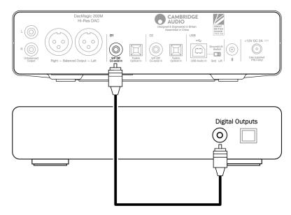
Connect your digital source to Digital Input 1 or 2. Either S/P DIF co-axial or TOSLINK optical types can be used. Optical is best to avoid ground loop noise, but some optical cables may not work correctly at 192kHz.
