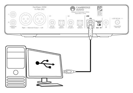
Class 2 USB Audio only. Windows based PCs require a Cambridge Audio USB driver to be installed before connection.
