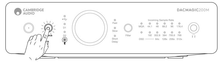
Selecting this allows the DacMagic 200M to receive wireless Bluetooth audio from most phones, tablets and laptops.
