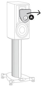
5 Tighten the three attachment screws (A) so that the loudspeaker is stable using the 5 mm Allen key. (B)
