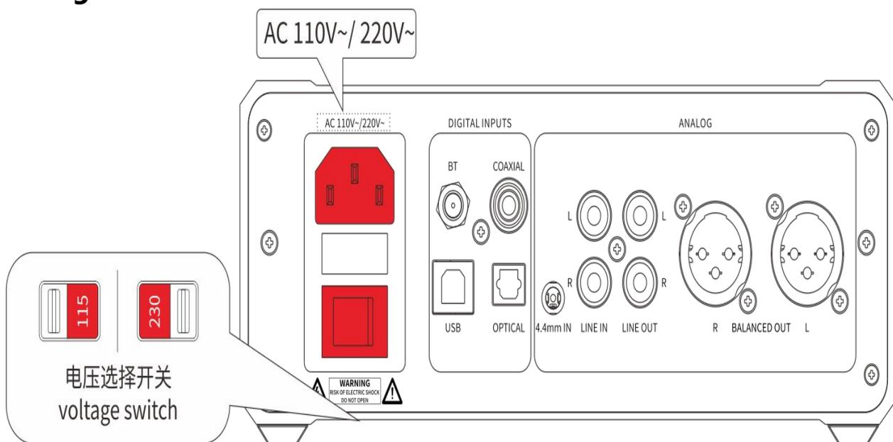
**B. Connect the source device to the K9 Pro and select the corresponding input source mode.**
