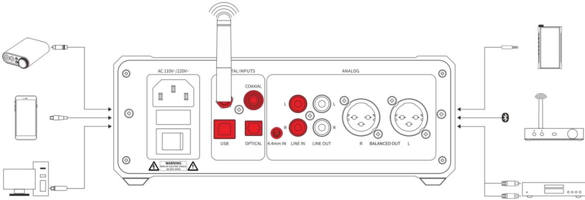
**C. Connect the K9 Pro to the output device and select the corresponding output mode.**
