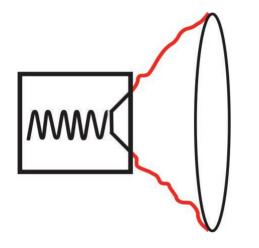
Conventional electrostatic headphones experience degradation of sound quality caused by the stator's interference.
