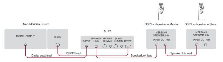
Use this application to connect a recent Meridian source with a SpeakerLink output to a pair of Meridian Digital loudspeakers that do not have SpeakerLink.
