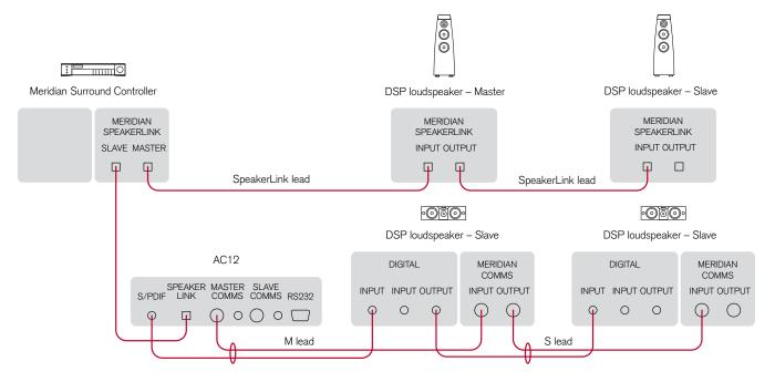
Use this application to connect up a multichannel system that includes both SpeakerLink and non-SpeakerLink loudspeakers, where the speaker you have chosen as the master does not have SpeakerLink.
