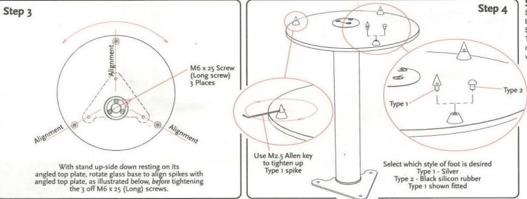
Step 4 Select from accessory box desired style of foot. Screw in place. Type 1 - Silver needs to be tightened with supplied Allen key.
