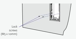
Once the frame is flush against the wall, lock it into place with the six M5 x 10mm button-head lock screws, and lock tight.
