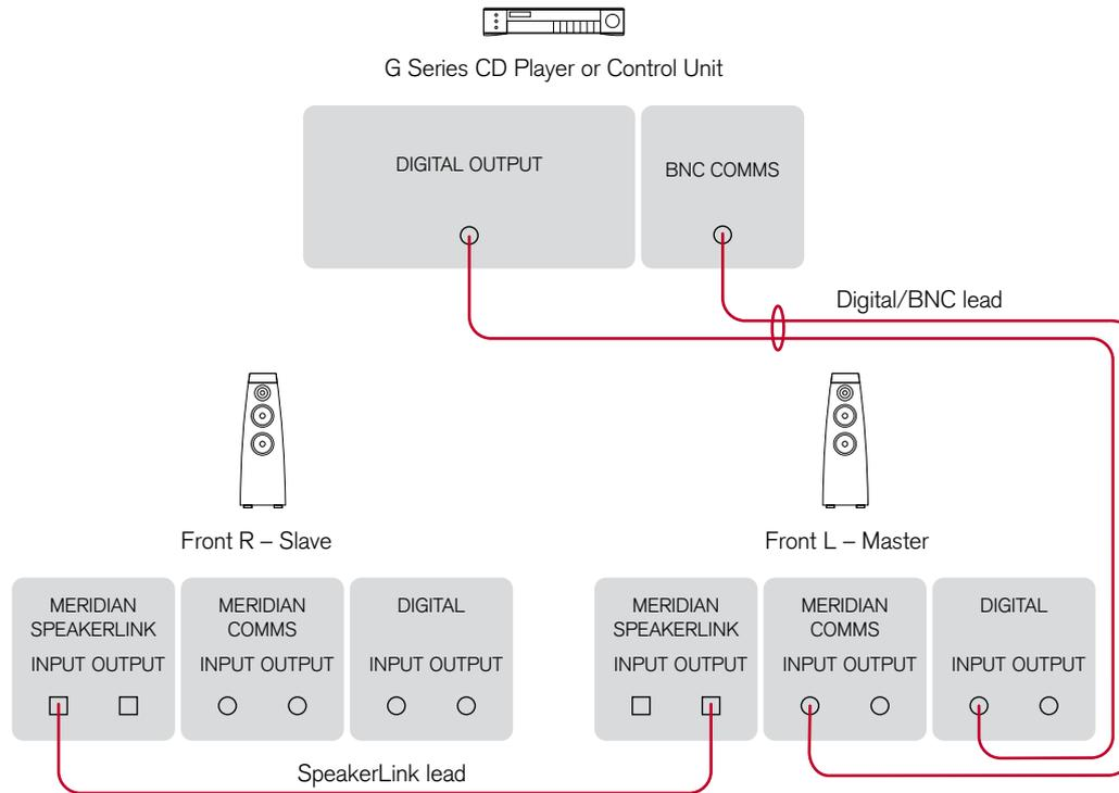
If the Meridian source or control unit provides a Meridian BNC Comms output, you will need to connect it to the DSP Loudspeakers using a Digital/BNC lead.
