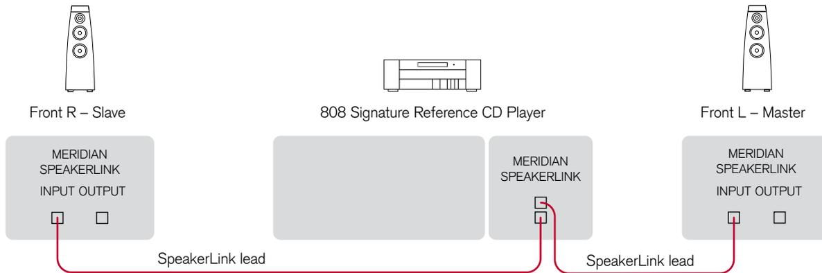
You can create a complete system by connecting a pair of DSP loudspeakers directly to a digital source. The DSP loudspeakers include volume, balance, and tone controls allowing you to control the system using an MSR+.
