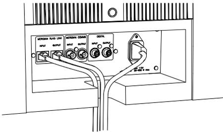
Finally refit the cover plate into position, concealing the input/output panel and connections.
