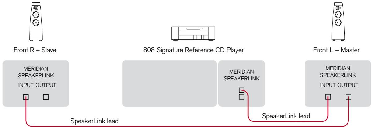
You can create a complete system by connecting a pair of DSP loudspeakers directly to a digital source. The DSP loudspeakers include volume, balance, and tone controls allowing you to control the system using an MSR+.
