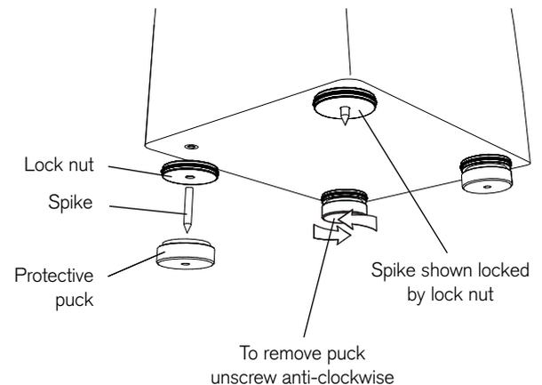
On carpeted floors all parts can be fitted and the spike should be adjusted so that it extends through the puck and penetrates the carpet pile to the floor underneath. Where a carpet has a deep pile you can fully unscrew and remove the puck to expose more of the spike.
