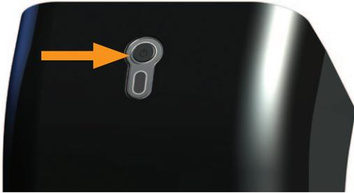
2. Press the Wifi input button (item 5 on Page 3) for approximately 12 seconds. The LED on the front flashes white (Pattern #3).
