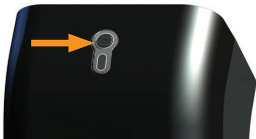
2. Press and hold the Wi-Fi input button (item 5 on Page 3) for approximately 12 seconds until the LED on the front flashes white (Pattern #3).
