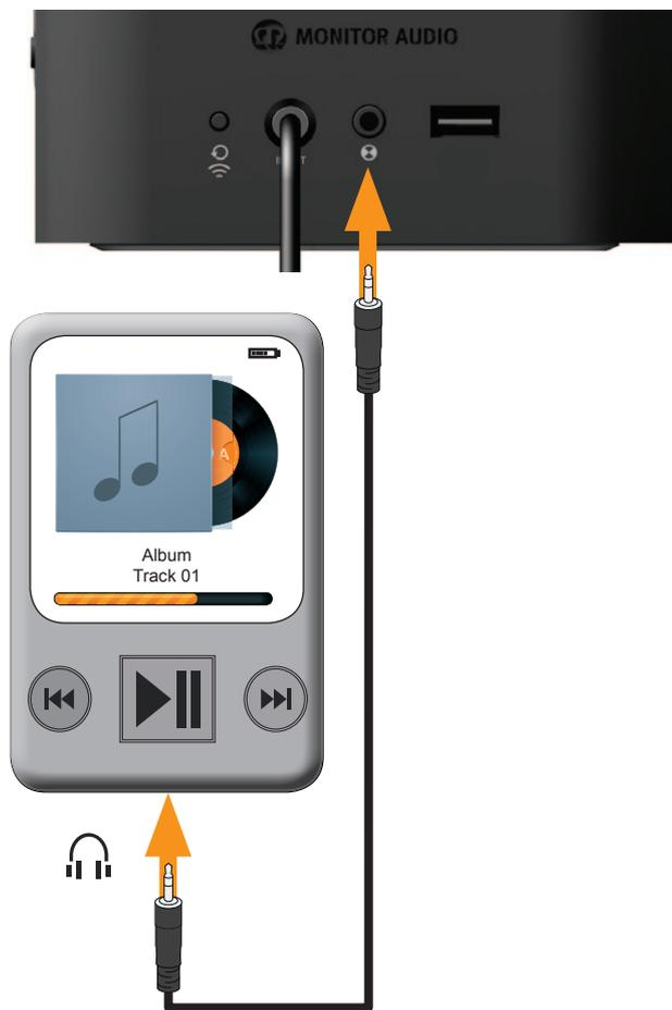
2. Press the Input toggle button on the S200 (item 6 on Page 3) until the Auxiliary source is selected (green LED).
