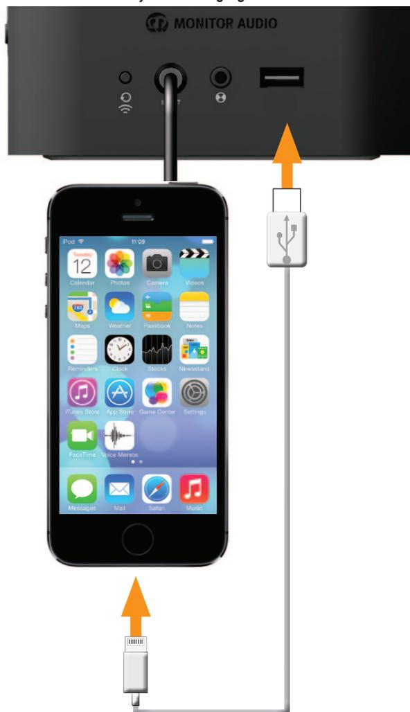
2. Press the Input toggle button on the S200 (item 6 on Page 3) until the USB source is selected (white LED).
