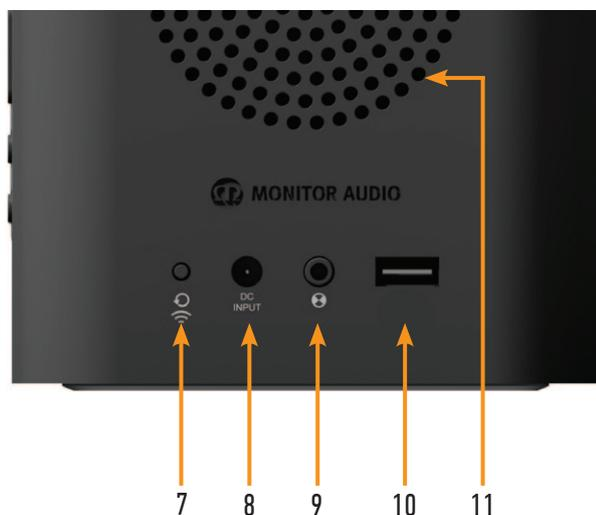
7. **Wi-Fi Sharing/ Factory Reset button.** This button also serves two purposes: A short press is required when connecting the S200 to a wireless network via the USB method. Press and hold for 12 seconds to perform a factory reset.
