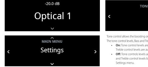
Press front panel [ $\checkmark$ ] button once for the Main Menu options to appear in the display. Use front panel a or s button to select through the Main Menu options – **Settings, Source Setup** and **System Info**.
