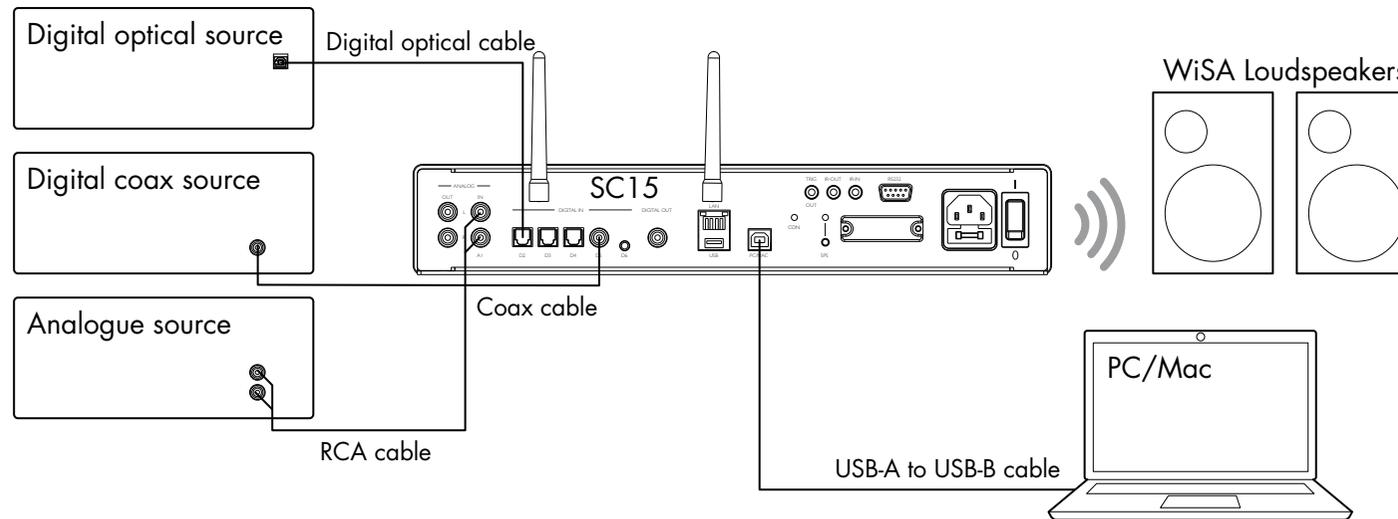
These methods of playing music from the SC15 involve connecting the source to the SC15 via a cable, and don't require Wi-Fi, Ethernet, or Bluetooth.
