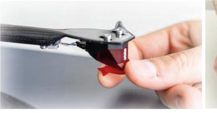
**16** Turn the front dial of the counterweight (not the whole weight) so the '0' is in line with marker at the back of the tonearm.
