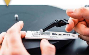
Balance the tonearm by turning the counterweight forwards and backwards on the rod.
