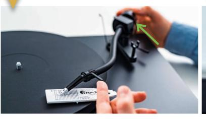
When the gauge stays level, your tracking force is set correctly.
