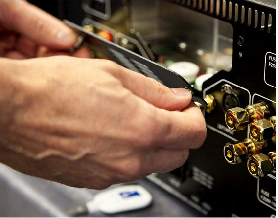
Remove the tube cover using Phillips screwdriver
