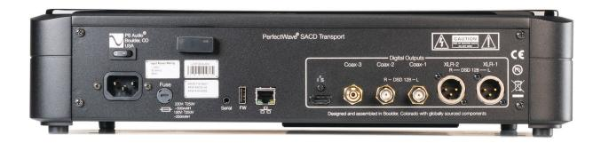
The stereo digital outputs of the PST can be transferred through three types of connections.
