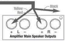
**NOTE:** The REL Arrow transmitter is equipped with internal circuitry to allow seamless connection to Class-D (digital) main amplifiers. If connecting to a Class-D amplifier, follow the above connection procedure for differential amplifiers.
