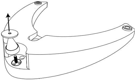
2.2 Slide the cable into the hole provided on the base as shown below (Insert the protective sheet (i.) between the base (a.) and the aluminum tube (b.)) :
