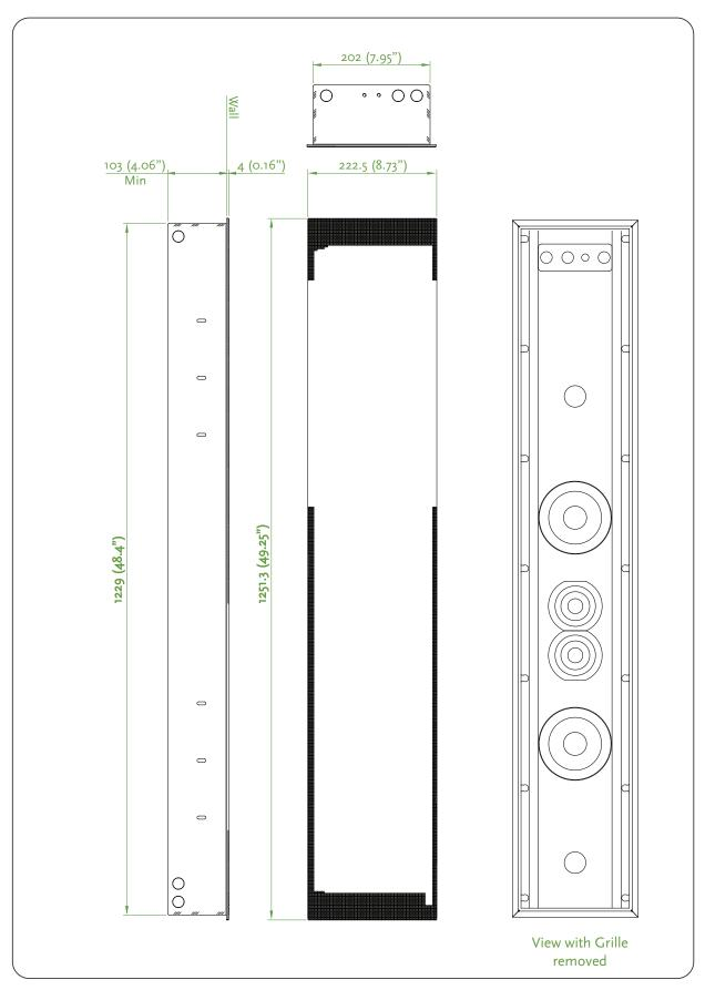
DSP640 Digital Signal Processing Loudspeaker
