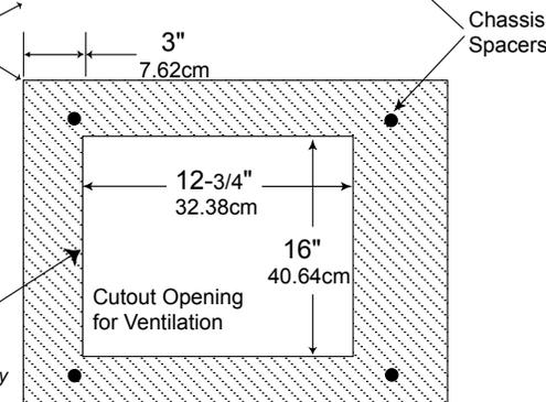
Note: Center the cutout horizontally on the unit. For purposes of clarity, the above illustration is not drawn to scale.
