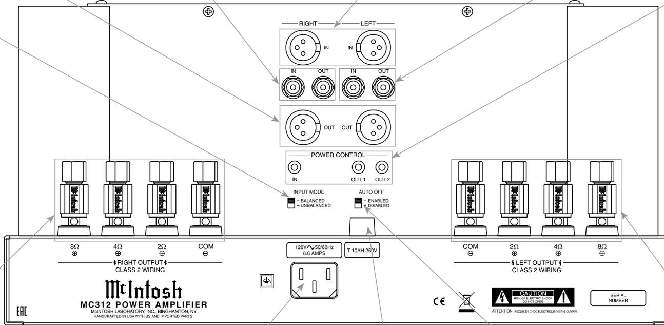
RIGHT OUTPUT Connections for a 2 ohm, 4 ohm or 8 ohm Loudspeaker
