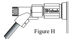
MC312 COM (Negative) Output Terminal and Positive Output Terminal indentified as 2Ω (ohms), 4Ω (ohms) or 8Ω (ohms) connection to match the impedance of the Loudspeaker, being careful to observe the correct polarities.
