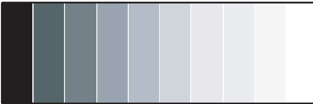
Figure 4-4. Typical Gray Bar Pattern for Adjusting Contrast
